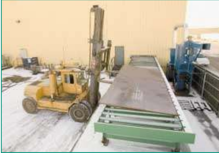
Load stock via fork truck outside the building.
