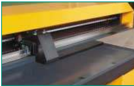
CNC gauging table for X and Y axis positioning.
