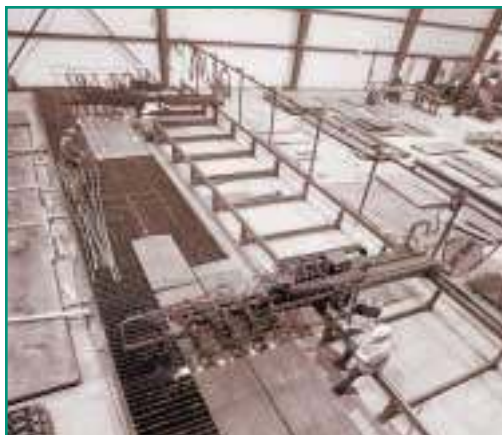
Typical burn table installations can occupy over 3000 square feet of shop floor space.
